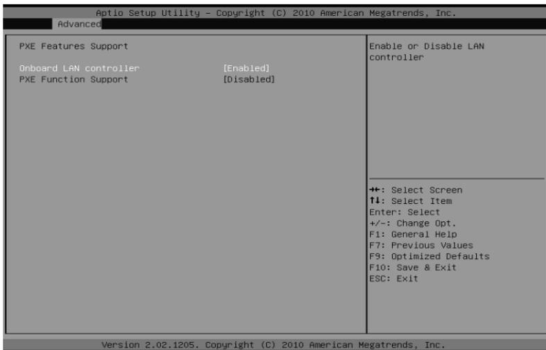
**Onboard LAN (板载网卡)**
